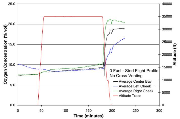
Figure 10. Zero Fuel Load Flight Test NEA Dispersion Data Without Cross Venting
