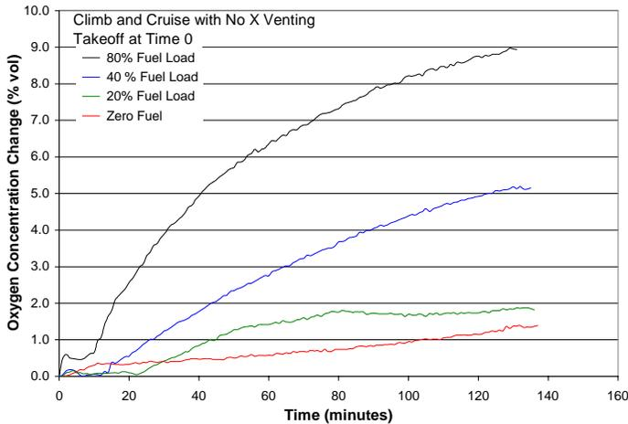
Figure 12. Average CWT O<sub>2</sub> Concentration Increase Comparison Plot for Different Fuel Loads
