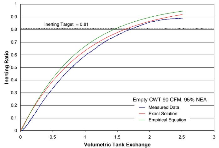
Figure 3. Ground Test 1 Nondimensional Ullage-Washing Data
