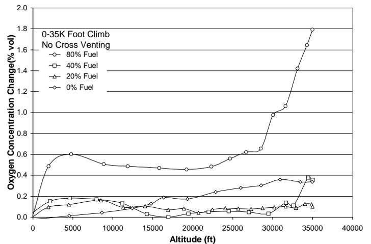
Figure 14. Change in Average CWT O<sub>2</sub> Concentration Comparison Plot for Different Fuel Loads During Climb
