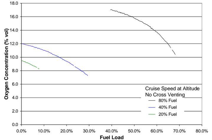
Figure 13. Change in Average CWT O<sub>2</sub> Concentration Comparison Plot for Different Fuel Loads During Cruise
