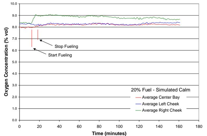
Figure 7. Twenty-Percent Fuel Load NEA Dispersion Data-Fuel After Inerting
