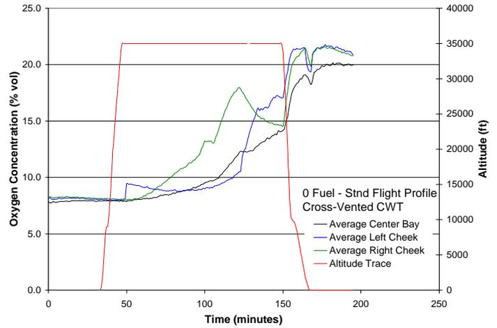
Figure 9. Zero Fuel Load Flight Test NEA Dispersion Data With Cross Venting Configuration
