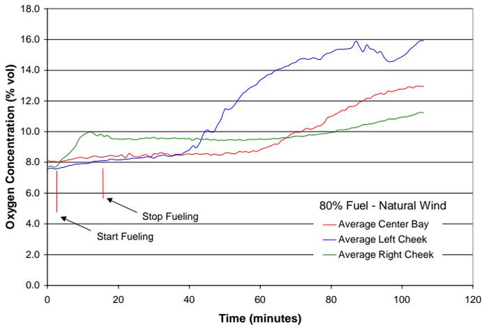
Figure 8. Eighty-Percent Fuel Load NEA Dispersion Data-Fuel After Inerting
