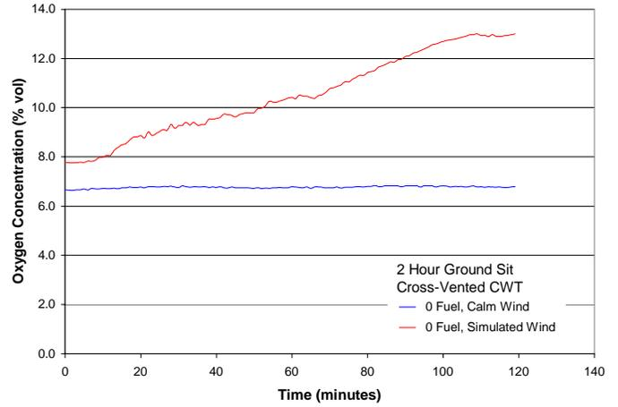
Figure 6. Comparison of NEA Dispersion for Two Wind Conditions
