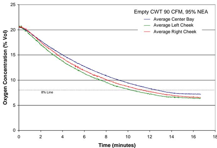
Figure 2. Ground Test 1 Ullage-Washing Average Oxygen Concentration Data
